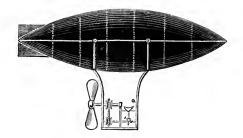
treadle mechanism, and a propeller, and the aëronaut is thus enabled to propel the balloon.
